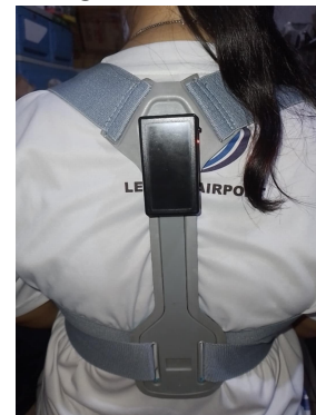
Fig. 5. Transmitter module at the back of the user.
