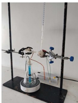
Fig. 2. Robotics-Assisted Acid-Base Titration Setup
