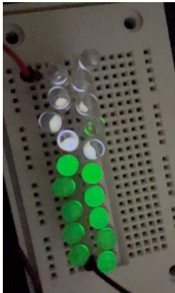
Fig. 8 shows the 19 LEDs in series light up during hand tapping.
