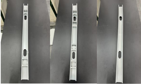
Fig. 9. Local buckling of samples with two holes and with stiffener: a) one-sided web; b) two-sided web; c) intermediate.
