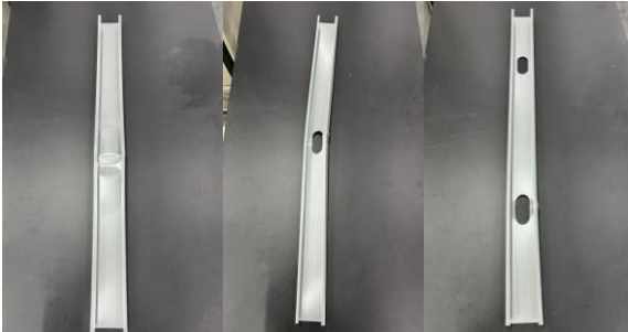
Fig. 7. Local buckling of samples without stiffeners: a) solid; b) one-holed; c) two-holed.
