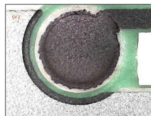
Figure 6. Overgrowth of PPy on a round carbon working electrode of the EP-PP chip when using 0.1 M pyrrole monomer for the electropolymerization solution
